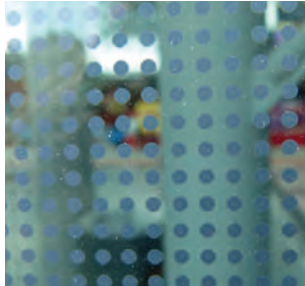
Fritted Glass Makes Windows Visible to Birds
